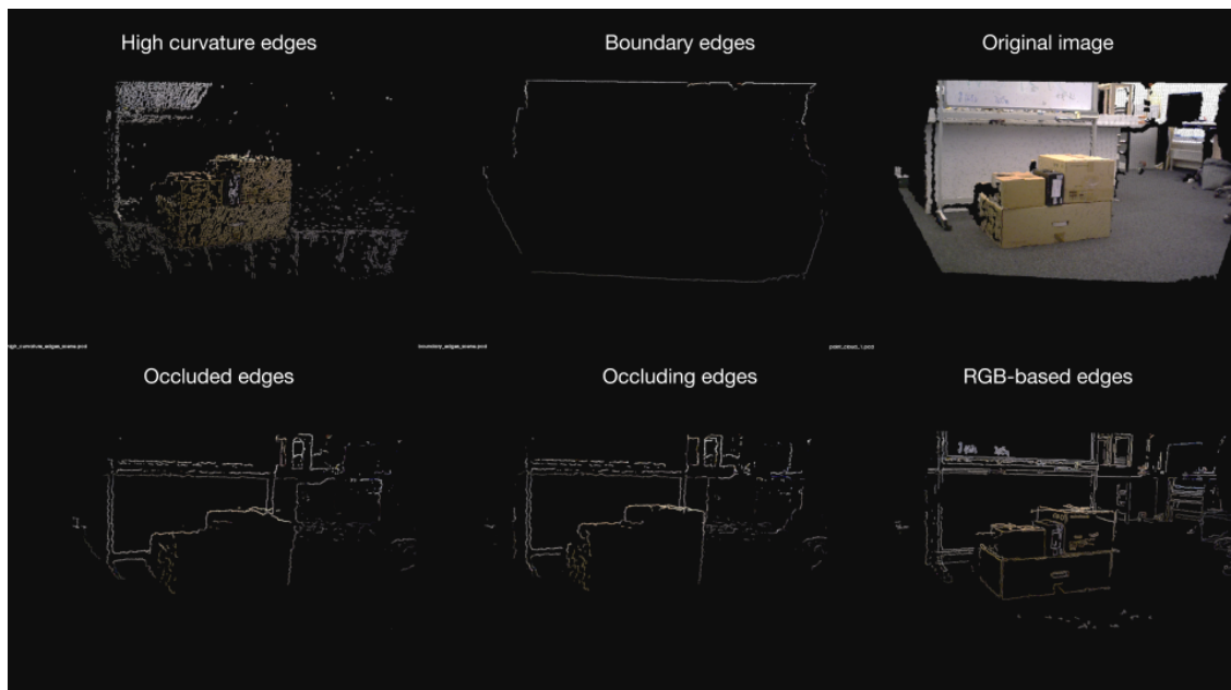
Figure 4.14: Detection of different edges types performed with OrganizedEdgeFromRGBNormals PCL class.
