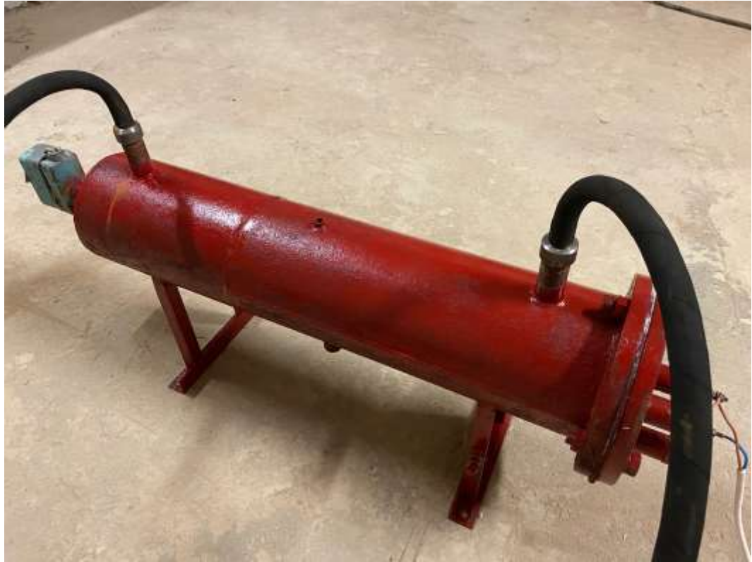
Figure 5.16 – Hot water boiler handmade
