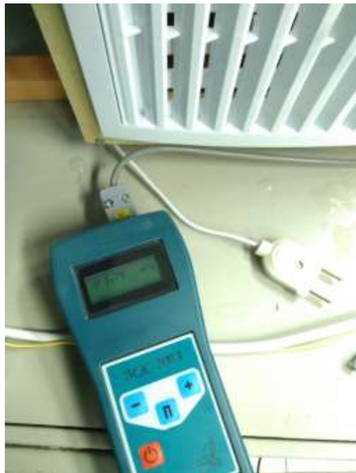
Figure 5.18 – Photo of the air flow speed reading on the MES-200A weather meter display
