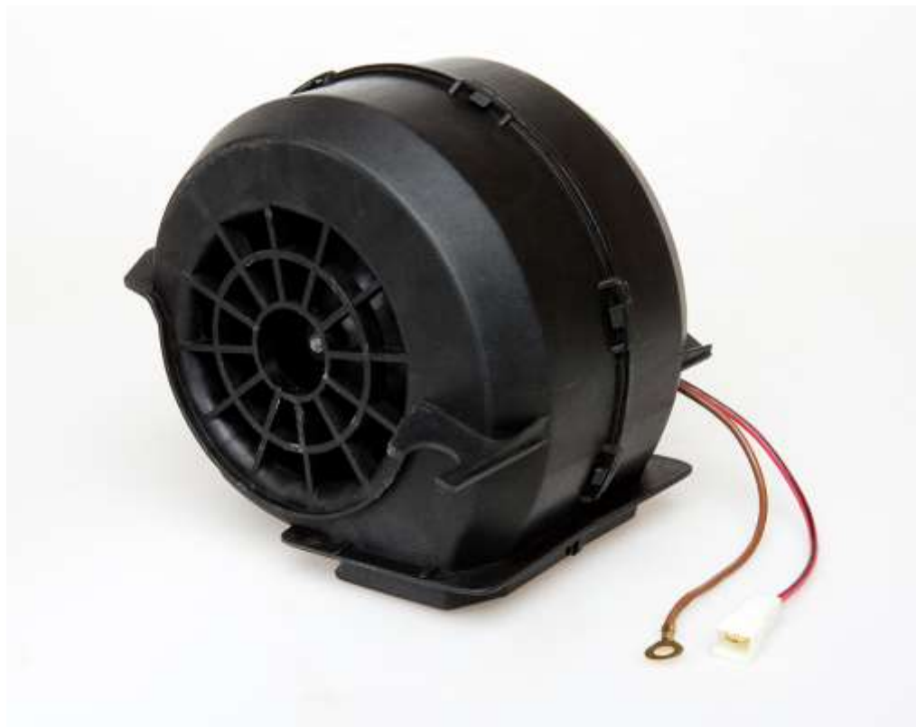
Figure 5.14 – VAZ 2108 stove fan
