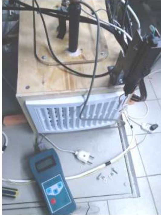
Figure 5.17 – Photo of the process of measuring the air flow velocity in the section of the experimental installation
