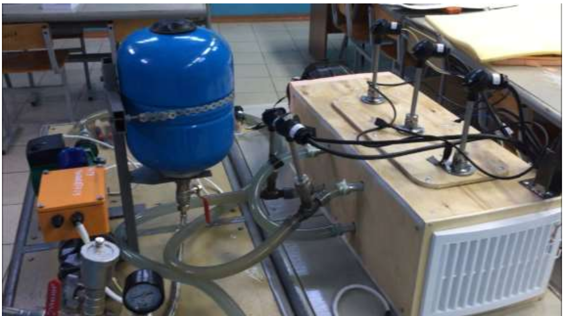
Figure 5.2 – Photo of the appearance of the heater unit and the complex, including a circulation pump, a hydraulic accumulator, a balancing valve and an electromagnetic fluid flow converter.
